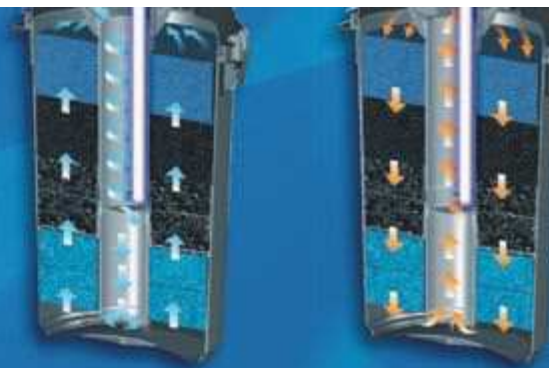
Normal Filter Operation Back Wash Operation
